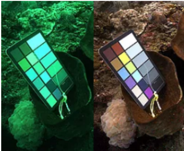
Fig. 4. Non-color corrected image on the left and image with Sea-Thru algorithm applied on the right
